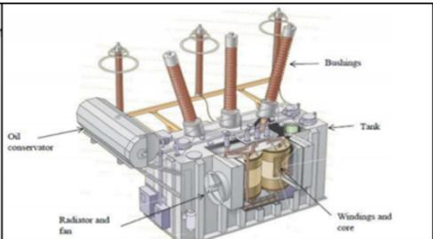
**Figure 5:** Compilation explaining the basic role of LPTs in the power grid and accompanied by an illustration of the parts and design of one type of extra-high voltage (EHV) LPT system. These graphics were assembled from a 2012 DOE document entitled: *Large Power Transformers and the U.S. Electric Grid*.
