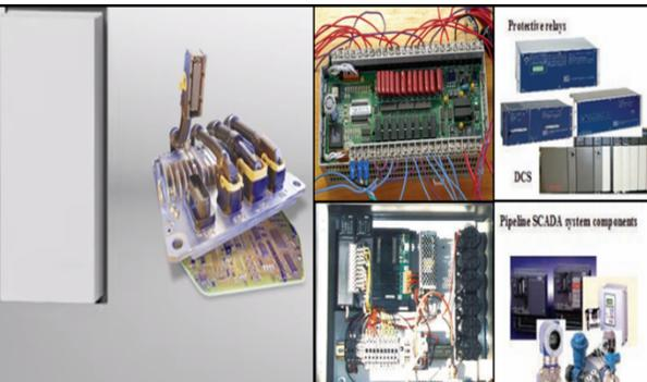
**Figure 13: (Left)** SafeDEC Digital Engine Governor by MTU Onsite Energy, used in EDGs in several nuclear power plants. **(Right)** SCADA systems tested by the EMP Commission in 2008.
