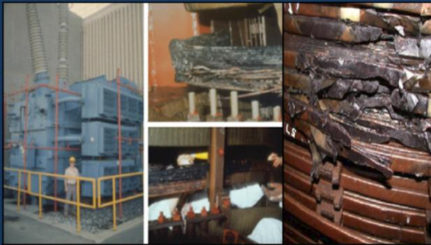
**Figure 6: (Right)** This is a picture of the Salem New Jersey Nuclear Plant GSU Transformer (~12mVA, 500/22kV single phase transformer) and permanent damage caused by the March 13, 1989 Geomagnetic Storm. Photos courtesy of PSE&G, and found in the 2008 EMP Commission Report. **(Left)** Similar damage has been observed on this transformer from South Africa.
